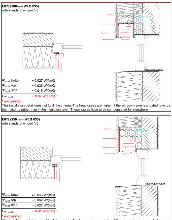
This installation detail does not fulfill the criteria. The heat losses are higher, if the window frame is situated towards the masonry rather than in the insulation layer. These losses have to be compensated for elsewhere.
