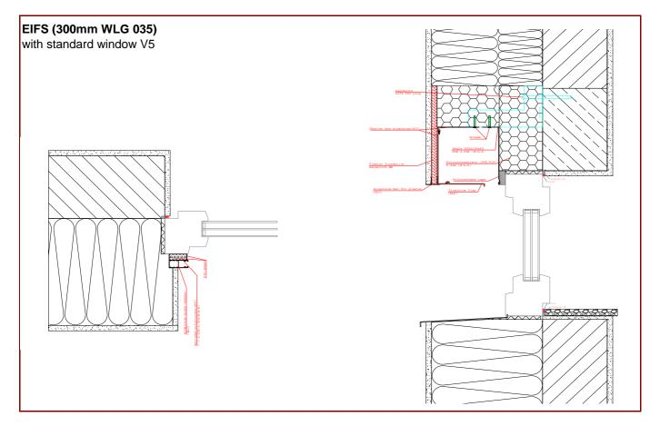
Installation based thermal bridge  $\Psi_{\text{instal.}}$  in Passive House suitable wall
